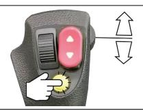
The roller on the outside right of the joystick activates the hydraulic connections on the boom head, at the same time as selecting the **ABC** button on the dashboard that determines which output is active. This button and its function are described further on in the manual.
