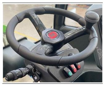
Use the steering wheel to guide the movement of the vehicle. A knob is provided to drive with one hand, keeping the other free for other controls.
