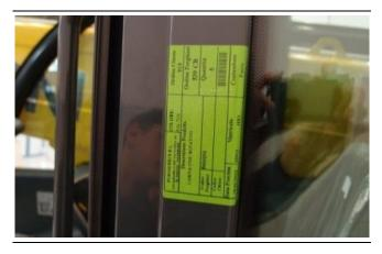
The cab identification plate is affixed on the jamb of the upper window, to the left of the driver.
