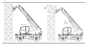
Put the vehicle perpendicular to the designated load. Make sure the forks pass under the load and are properly adjusted to the load.
