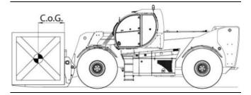
Never try to lift loads heavier than the rated capacity of the vehicle.
