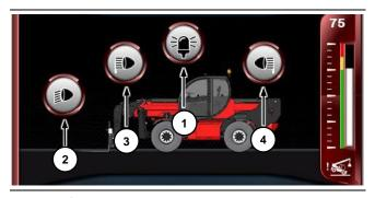
Button ① activates the orange beacon that indicates that the vehicle is in motion. Buttons ②, ③ and ④ activate the lights at the top of the boom, those on the front of the cab and those at the rear of the cab, respectively.
