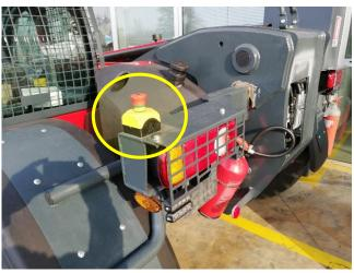
The THU version has two additional emergency stop buttons (in addition to the standard one inside the cab, on the dashboard to the right of the driver's seat). The additional buttons are located one on the right front mudguard and one on the left rear mudguard.
