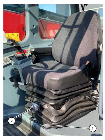
Use the lever (1) to move the entire seat structure in the longitudinal direction including the right armrest and relative joystick.
