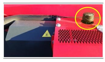
To top up the oil level, open the cap at the top of the tank. Pour oil of suitable strength up to the correct level.
