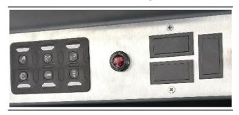
There is also a warning light inside the cab, in the front right-hand area below the windscreen, that visually indicates the vehicle's movements to the operator in real time following the logic of the additional front LED lights.
