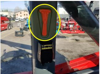
The rear window also serves as an **emergency exit**. To open it, follow the procedure described above. If it is not possible to exit through the rear window, there is a **RED hammer** on the right door jamb of the cab; it must be used (in the event of an emergency) to break the glass of the cab to facilitate the driver's exit. *Contact your dealer to have the glass replaced*.
