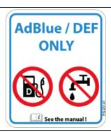
This sign is positioned near the AdBlue® tank connector.
