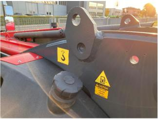
The vehicle is provided with four lifting points, in the front part of the chassis and in the rear part, all marked by a yellow sticker as shown above.
