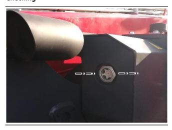
The hydraulic oil tank is on the left side of the vehicle. Check the hydraulic oil level through the inspection window at the back of the tank.
