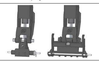
The "I" coupling (patented by MAGNI TELESCOPIC HANDLERS Srl) is designed to be more rigid, more compact, and easy to fit, in comparison with those of competitors and is intended solely for equipment designed and constructed by MAGNI TELESCOPIC HANDLERS Srl with a similar coupling.
