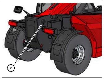
Lubricate pin ② injecting grease in both grease nipples present on the boom.
