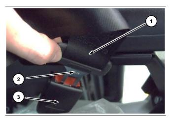
The seat belt is provided with an automatic winding system. The system is blocked automatically if the belt is pulled violently.
