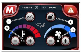
The controls for the cab air conditioning system are at the top of the controls page.
