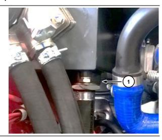
Open the engine compartment bonnet and place a funnel, connected to a fluid recovery tray on the floor, under the threaded drainage cap (1), indicated above.
