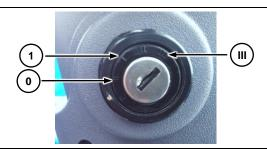
The starter switch is located on the right-hand side of the steering column. The switch has three active positions:
