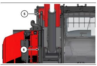
Lubricate pins (5) and (6) of the compensation cylinder. To make access to the grease nipples easier, lift the telescopic boom completely.
