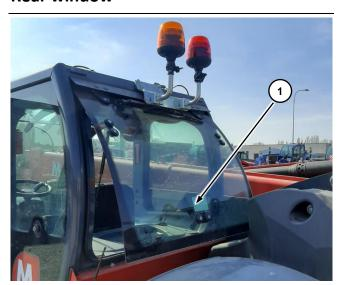
The rear window of the cab can be opened to allow natural ventilation. To open the window, only from inside the cab, turn handle ① anticlockwise to unlock it. Push the window outwards. To shut the window, pull it inwards by means of lever ①. Turn lever ① clockwise to lock the window shut.
