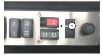
Press and hold down switch ①. Retract and lower the boom to check the correct working of the emergency hydraulic pump.
