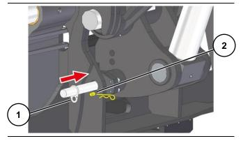
Take the shear pin ① from its housing and insert it in all the way, taking care to align the hole. Complete the procedure by inserting the split pin ② in the hole to prevent the shear pin from coming loose accidentally.
