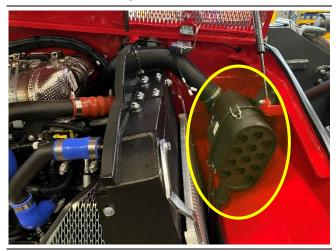
Unclip the catches and remove the front filter cover.
