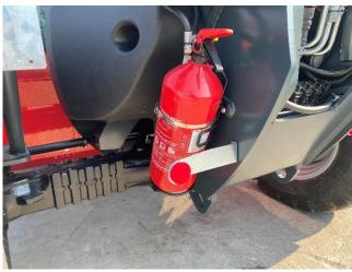
The THU version is equipped with 2 fire extinguishers, each with a capacity of 6 kg, located respectively on the front left side (in front of the cab) and on the rear left side (behind the thermoplastic fuel tank) of the vehicle.
