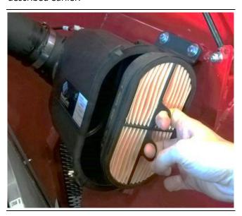
Hold the filter element with two fingers in the holes and pull to separate it from its seat.
