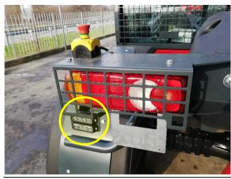
The THU version is equipped with directional lights, located below the front and rear lights.
