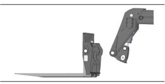
Bring the vehicle perpendicular to the equipment with the boom completely retracted and lowered. Retract the slewing jack to make hooking easier. Stop the vehicle with the quick-fit coupling about a metre away from the equipment. Move the reverse gear lever to the neutral position and apply the parking brake.
