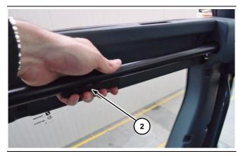
To open the cab door from the outside, pull outer handle ②, then hold the door all the way. The cab door must be kept closed when the vehicle is in operation. To allow natural ventilation inside the cab, use the rear window or side window.
