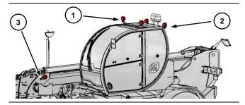
The vehicle can be fitted with additional lights to light up the work area. The additional work lights are divided into three groups:
