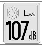
The plate indicating the acoustic power level emitted (guaranteed), according to the Noise Directive 2000/14/EC, is affixed inside the cab on the panel to the right side of the steering column, next to the vehicle's identification plate.
