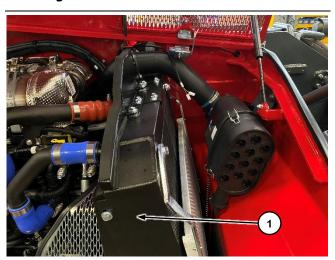
To remove dust and debris from the radiator mass ①, compressed air, pressurised water or steam can be used. However, it is preferable to use compressed air.
