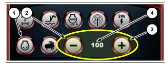
This selection ① makes it possible to activate, for a certain accessory, the continuous movement of one of its element such as a mixer bucket, adjusting the operating speed by means of the buttons concerned, ② and ③.
