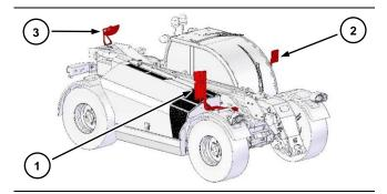
The vehicle has five rear view mirrors supplied as standard: three on the right side of the chassis  $\bigcirc$ , one on the left side of the cab  $\bigcirc$  and one on the rear
