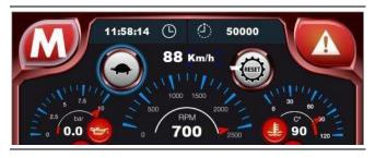
the AdBlue® liquid level, the engine rpm counter and coolant temperature for D7 (Tier4f / Stage V) engine as shown in the graph below.
