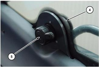
To shut the window, turn lever (5) anticlockwise to release the limit stop block. Hold the window by means of handle (2) till it is completely closed. Turn lever (1) clockwise and make sure the window is locked in the closed position.
