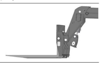
Extend the telescopic boom slowly, checking the alignment, then raise it to fit the accessory. Raise the equipment by a few centimetres off the ground to ensure the elements fit in perfectly.
