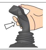
To impart commands using the joystick, press and hold the manoeuvre enabling button under the joystick as shown above, making sure that the joystick is in a neutral, central position.
