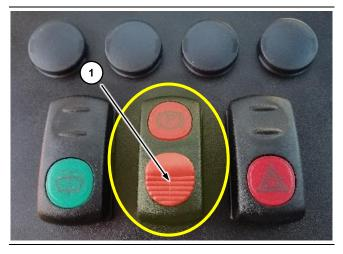
The switch for engaging/disengaging the parking brake is under the steering wheel in the centre of the steering column. Press the upper part of the switch to put the parking brake on. Check to make sure the indicator light in the main page of the multiple function display lights up.
