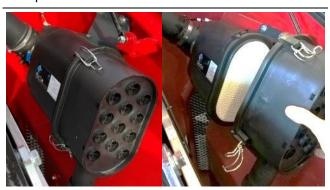
Grip the filter housing and remove it from its seat.
