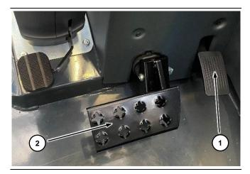
Press the accelerator pedal ① to increase the engine speed.
