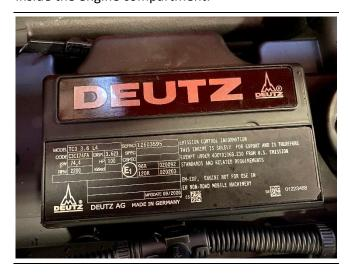
Depending on the engine installed, it may be barely visible because it is obstructed by the engine's after-treatment devices. In such cases a duplicate identification plate is affixed in one of the two areas described below.
