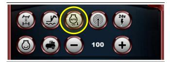
The button indicated is used to activate or deactivate the engine speed electronic control function: if selected, as soon as a hydraulic movement is imparted to a forklift truck component, the engine automatically increases the speed to provide force to the services pump and consequently facilitate the movement imparted.
