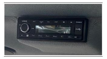
The vehicle radio is present on the rear covering of the cab behind the operator's head. The speakers are present between the driver's seat and the rear window. The radio is included in the standard vehicle supply. However, any other radio can be fitted with dimensions 1-DIN in accordance with standard ISO 7736. For operation of the radio installed, refer to the Instruction Manual included in the package delivered with the vehicle.
