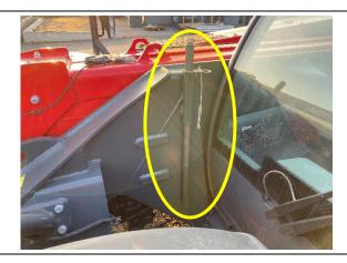
The housing of the shear pin for the quick-fit coupling of the equipment is present in the front part of the vehicle chassis. The shear pin must also be present on the vehicle so as to be available when required. Always fit the shear pin in its housing when not in use.
