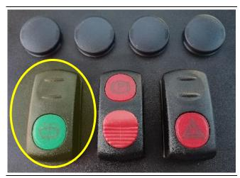
To activate the washer liquid supply on all the nozzles, press the bottom part of the green button on the left of the steering column under the steering wheel.
