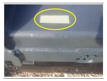
The vehicle's serial number is shown on the FRONT RIGHT SIDE of the chassis.
