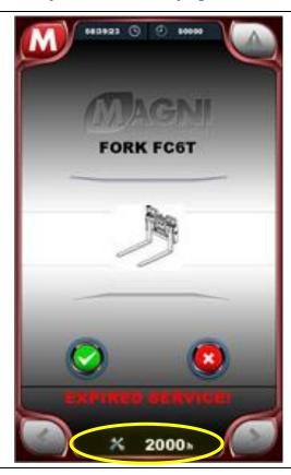
This page is displayed every time the sensor at the head of the telescopic boom detects new interchangeable equipment. This page cannot be selected manually.
