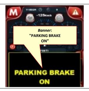
The parking brake can also act as an emergency brake, therefore there is no logic related to the forward speed that prevents it from being engaged.
