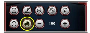
Press this button to activate/deactivate the compressed air outlet.
