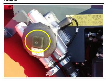
Park the vehicle on a flat surface: clean the filter housing and surrounding areas to prevent dirt from entering the circuit. Unscrew the cover.
