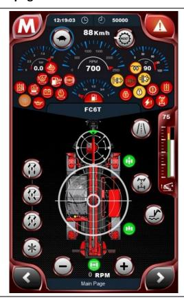
The main page groups together the main information of the vehicle in the driving on wheels configuration. For all the models the display shows, at the top: the daily time and working hours of the forklift truck, the speed selection button and the reset button.
