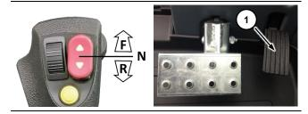
The status from parking brake on to parking brake off switches smoothly without any forcing on the mechanical brake of the axle even on steep slopes. This function is always associated with pressing the button in the centre of the steering column.
