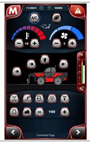
The controls page contains information and controls regarding the cab conditioning system and control buttons for the work lights, boom suspension and radio control.
