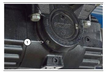
Set the vehicle in the parking position. Make sure no one approaches the work area. Stand near the front axle oscillation bushes. Inject grease in the grease nipples ① present on both sides of the axle (front and rear).
