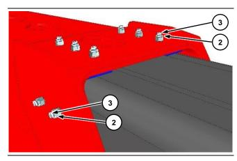
Loosen all the lock nuts ② of the upper and side sliding blocks at the top of the boom. Screw all the grub screws ③ all the way without tightening them, then unscrew them all by half a turn.
