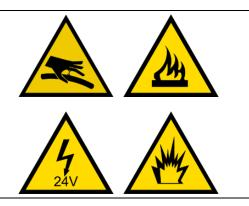
The safety symbols shown in the figure are applied inside the engine compartment on the right.
