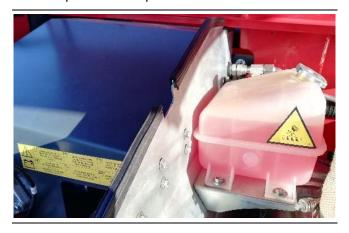
The level is correct when it is halfway between the MIN and MAX marks.
