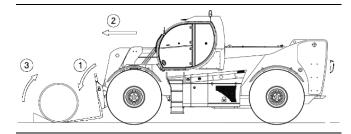
Position the vehicle at right angles to the load. Approach the load with the telescopic boom completely lowered and retracted. Apply the parking brake and set the reverse gear lever in neutral. Incline the quick-fit coupling downwards ①. Extend the telescopic boom slowly ② and at the same time rotate the quick-fit coupling upwards to insert the forks under the load ③.
