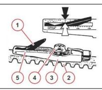
To check the tension of the belts, lower the arm of indicator 1 in the tester.
