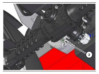
Unscrew the filler cap. Place a suitably sized container under the fuel tank near drainage cap (2).
