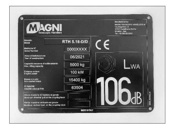
The new version of the identification plate is not only made with a different technology (laser marking instead of dot marking), but it also includes information on the (guaranteed) sound power level according to the Noise Directive 2000/14/EC. The data shown are the same as those on the identification plate valid up to October 2021.
