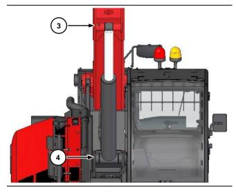
Lubricate pins 3 and 4 of the lift cylinder. To make access to the grease nipples easier, lift the telescopic boom completely.
