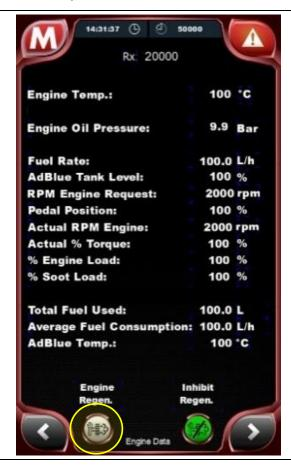
This automatic function can be disabled by the user for operating requirements (e.g. instructions from the site manager, work in closed areas where this operation is strongly advised against, such as tunnels or warehouses) by pressing the green button indicated.
