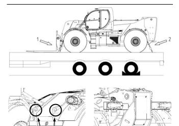
Install anchoring devices approved for the weight of the vehicle with equipment. Fix the anchoring devices at the four designated points ① and ② marked with the following symbol.
