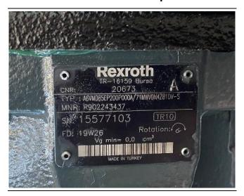
The transmission identification plate is affixed on the hydrostatic engine, inside the engine compartment, on the right side of the vehicle.
