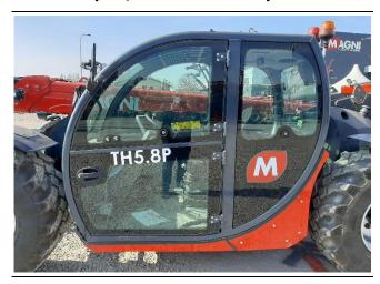
The handler has a cab, consisting of a welded steel structure enclosed by glass in accordance with European Regulation UNECE R43. The front window acts as a windscreen and is therefore approved for driving on public roads (where permitted). The rear window (which can be opened) also serves as an emergency exit. The cab contains:
