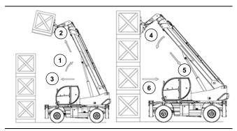
After picking up the load, lift 1 and extend 2 the telescopic boom to position the load above the area in which it is to be deposited. Move the telescopic handler close to the area where it is to be deposited 3.
