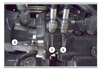
Move under the vehicle near the front axle from the right side. Identify the hydrostatic transmission and hydraulic actuator of the reverse gear.
