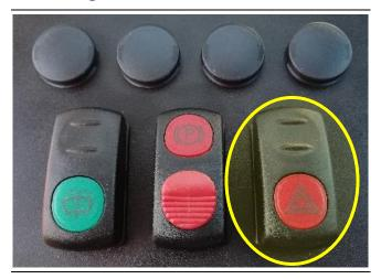
The switch for activation of the hazard lights is on the right hand side of the steering column, under the steering wheel.
