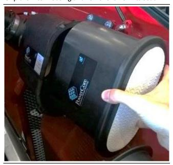
Wipe thoroughly inside the filter housing with a damp cloth. Avoid the use of aggressive solvents or products as these can damage the safety filter or the filter housing.
