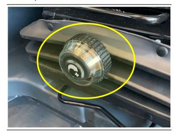
Turn the graduated grey spring suspension adjustment handle on the seat to adjust its preload until the number in yellow approximately matches the weight of the operator.
