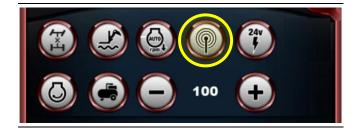
To operate the forklift truck externally using radio control the receiver connection present on the vehicle must be activated by pressing the button shown above.
