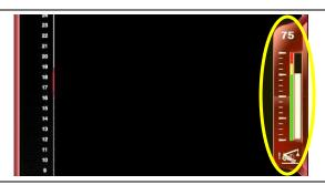
The load percentage indicator in combination with the load chart provides complete clear information regarding the operating conditions of the vehicle.
