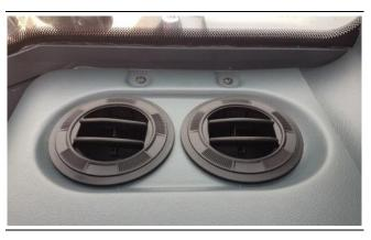
The air vents positioned in front of the driver, behind the seat, and on the left upright let in air flow into the cab. Each air vent can be opened and closed, and is used to adjust the direction of the air flow.
