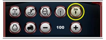
Press this button to activate the power socket (optional) present at the top of the boom for supplying current to the accessories that may be fitted.
