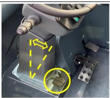
To adjust the inclination of the lower part of the steering column, while correctly seated in the driver's seat, press the pedal shown in the photo and pull the steering wheel towards you; once you have found the correct position, release the pedal.
