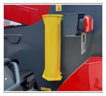
The device must be fitted on the piston rod and locked in place by operating the lifting cylinder.
