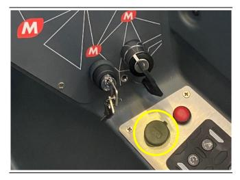
A USB socket is present under the multiple function display with a dialogue function with the software installed on the vehicle to help quickly update.
