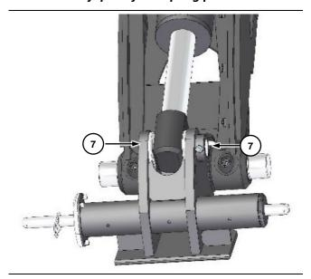
Lubricate the pin of quick-fit coupling ⑦ through the grease nipples.
