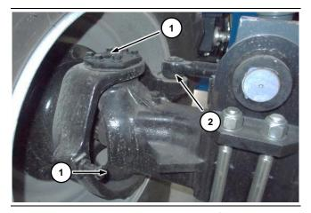
Lubricate the wheels rotation pins ① by injecting grease in the grease nipples provided for the purpose. Remove the excess grease. Lubricate the ball joint ② injecting grease in the grease nipples provided for the purpose. Remove the excess grease.
