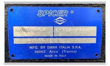
The axles identification plate is affixed on the top of the differential.
