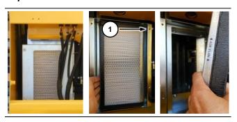
Open the compartment in the rear part of the cab to access the filter housing.
