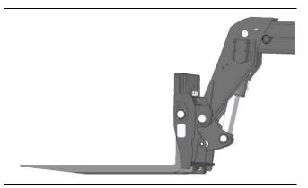
Rotate the quick-fit coupling until it is aligned perfectly with the accessory.
