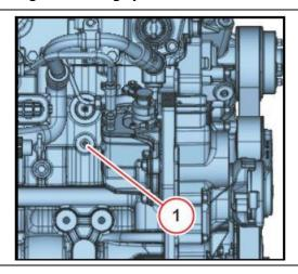
Set the vehicle in the parking position. Remove the radiator cap carefully to release the residual pressure. Place a suitably sized container under the drainage cap to collect the coolant flowing out.
