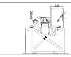
In case of irregular loads, determine the centre of gravity in the transverse direction to the vehicle before making any movement.
