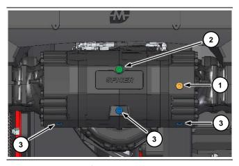
Remove level cap ①. The oil must flow out through the opening.
