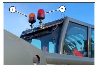
The **ORANGE** work light (1) can be switched on while the vehicle is running to indicate movement. It is mandatory to use within the construction site areas and in the cases indicated for driving on public roads.
