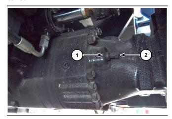
Go under the vehicle near the front axle. Unscrew lock nut ① of power screw ②. Tighten the power screw completely. Tighten it further through another turn to deactivate the negative control brake. Repeat the operation for both screws on the same axle.
