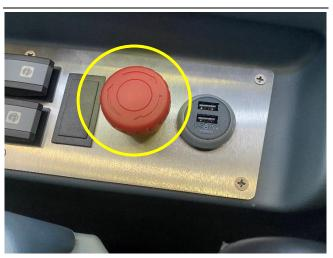
Press the emergency stop button to stop the engine and interrupt all vehicle movements.
