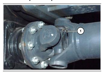
Set the vehicle on a flat surface in the parking position. Make sure no one approaches the work area. Lubricate the universal joints by injecting grease into the grease nipples ①. Repeat for all the transmission shaft joints. Remove the excess grease.
