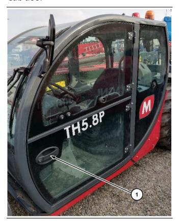
Open the cab door lock using the key meant for the purpose. To open the cab door from the outside, pull outer handle  $\bigcirc$ 1, then hold the door all the way.
