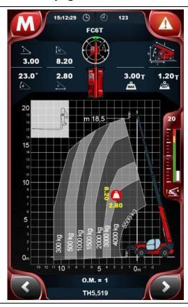
The load control page contains information regarding the configuration of the telescopic boom and equipment fitted.
