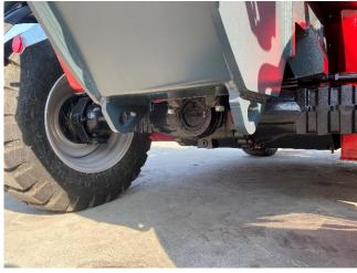
The vehicle is provided with four anchoring points, in the front part of the chassis and in the rear part, all marked by a yellow sticker as shown above.
