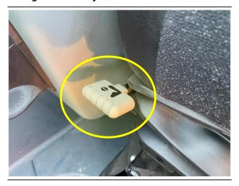
Use the grey lever (when seated) to the right of the seat to change the inclination of the seat surface to your liking.
