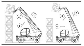
If possible, lower the load without moving the forklift truck. Lift the boom to move the load away (3), retract the telescopic boom (4) and lower it to bring the load to the transport position (5).
