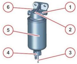
1 pump fuel supply - 2 bleed screw - 3 electric connection for the water level sensor - 4 drainage cap - 5 filter cartridge - 6 fuel tank inlet.
