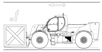
Manually adjust the width of the forks so that these can be inserted in the openings in the pallet at the base of the load. If there is no pallet, assess the width of the blades to give the load maximum stability.
