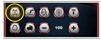
Pressing this button disconnects the drive to the rear axle wheels.
