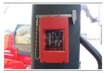
The container for the keys used for disconnecting the safety systems is fitted on the left jamb inside the driver's cab.
