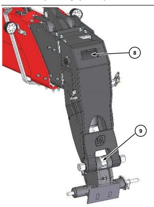
Lubricate pins **(3)** and **(9)** of the slewing cylinder by means of the grease nipples provided on the cylinder.
