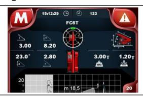
The section at the top of the load control page contains information regarding the boom configuration. The data shown in the graph above and organised from left to right, top to bottom, are:
