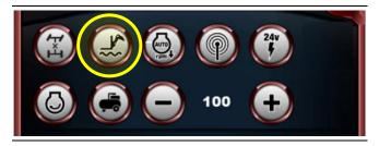
This button is present if the optional concerned is present on the forklift truck being used. The telescopic boom suspension is designed for operating the vehicle on uneven ground with loads raised.
