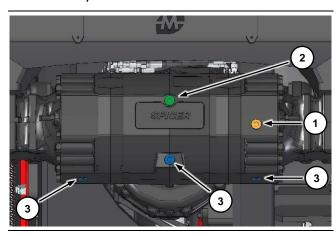
Remove the three drainage caps of the differential **3**. Wait for the oil to drain completely out of the differential. To speed up the operation, remove filler cap **2**.
